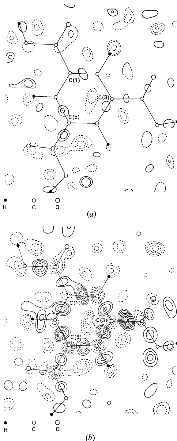
Fig. 3. Difference maps through the best plane of the molecule. (a) \Delta\rho(X) map generated with X-ray parameters. (b) \Delta\rho(N) map generated with neutron parameters. Positive and negative contours are shown as unbroken and broken lines, respectively. First contour at 0.10 \text{ e } \text{\AA}^{-3} . Contour interval: 0.05 \text{ e } \text{\AA}^{-3} .
